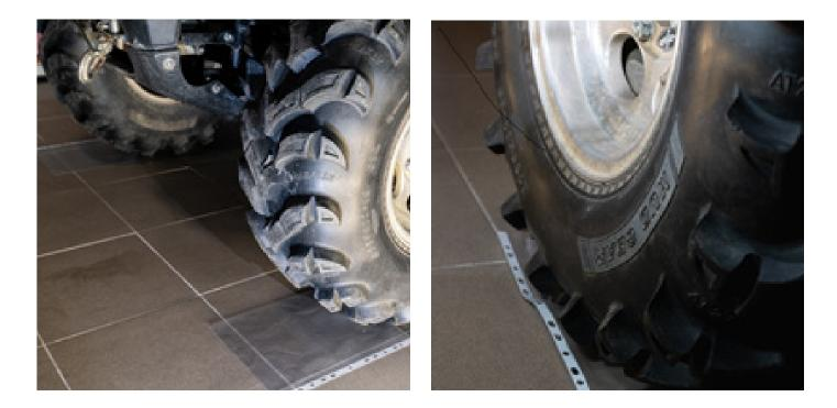
**4** Set the steering wheel to the middle position! Use a tape measure, you can measure to any symmetrical point.
