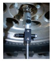
**6** If the wheel camber is specified in the geometry data and is adjustable, measure the value with the protractor and set it as described in the service manual.
