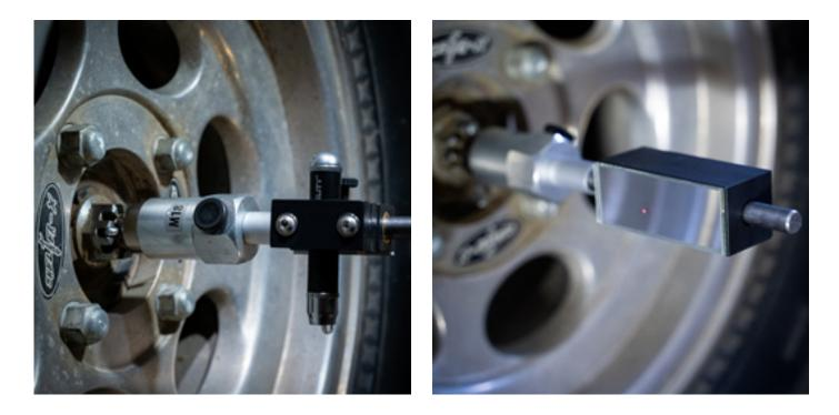
**11** Light to the mirror console. Reflect the light back onto the scale of the laser module. Find the center of the scale with the adjustment screw of the toe connecting rod. Then the front wheel runs "straight".
