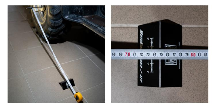
**13** You can then adjust the geometry by adjusting the length of the connecting rod. If the light travels inwards from point "0", you measure spread, if it travels outwards, you measure cohesion.
